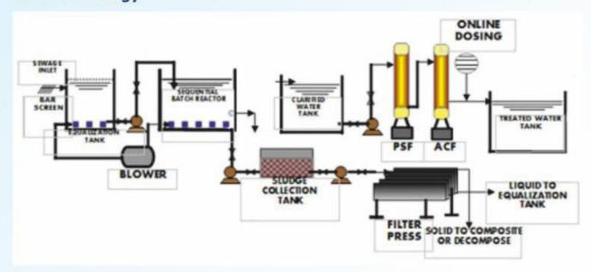
The Sequencing Batch Reactor (SBR) is a fill-and draw activated sludge system for wastewater treatment. In this system, wastewater is added to a single "batch" reactor, treated to remove undesirable components, and then discharged. Equalization, aeration, and clarification can all be achieved using a single batch reactor. To optimize the performance of the system, two or more batch reactors are used in a predetermined sequence of operations.
